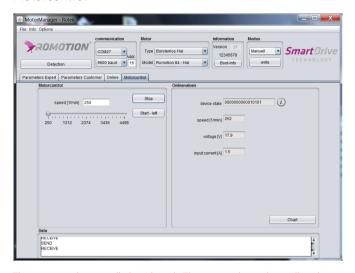
The motor can be controlled via this tab. The rotational speed as well as the direction of rotation can be specified. Furthermore, the current state of the motor is displayed in the field "Onlinevalues" on the right side of the window.
