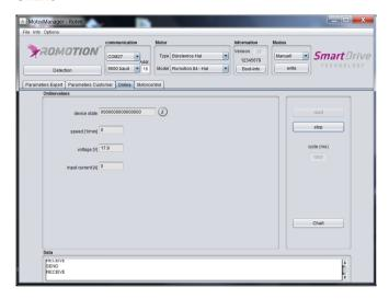
This tab is used for live monitoring of the motor. By clicking on the "read" button, the current status of the motor is read in regular intervals and displayed in the left-hand window. This can be stopped via the "Stop" button. The parameter "cycle" is used to set how often a new value should be read. The minimum value is 100 ms.
