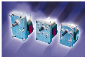
Shaded pole motors are used as low-cost A/C motors at low outputs where a high starting torque is not necessary. They only have one stator coil and do not need an expensive capacitor that is subject to wear, making them sturdy and durable. . ROTEK has been selling these motors in the German-speaking region since 2003.
