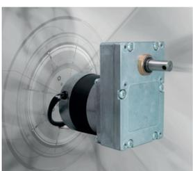
It allows torque of up to 15 Nm in continuous operation and 20 Nm at peak loads. With gear ratios of  $i=30:1$  to  $i=3000:1$ , speeds of 50 to 0.33 Upm can therefore be achieved.
