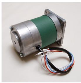
Its advantage compared to electrical and mechanical brakes is the complete absence of wear and tear and its reliability. Additionally no extra electrical connection is necessary for the brakes. It has the same diameter as the motor and is thereby only 22mm longer. This is another advantage if only limited installation space is available. Its holding torque is 6 Ncm.
