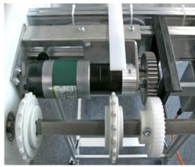
The modular construction of the main components - straight, angle and Z moulds - allows virtually any adjustment to the respective area of application. Gear motors provide the drive, and are housed inside the module body. While beforehand simple spur gear motors were applied here, for around a year the transportation technology specialists from Swabia have been using the synchronous motors of the Rosync range from a small motor manufacturer from Bremerhaven - Rotek.
