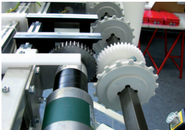
Using the energy saving motor to drive a link belt conveyor, as shown here, renders conveyor design extremely compact
